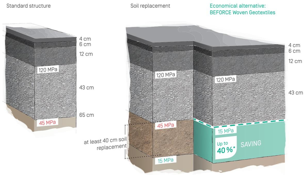
With BEFORCE Woven Geotextiles, the costs of at least 40 cm of excavation and disposal and of the delivery and installation of replacement material are saved.
