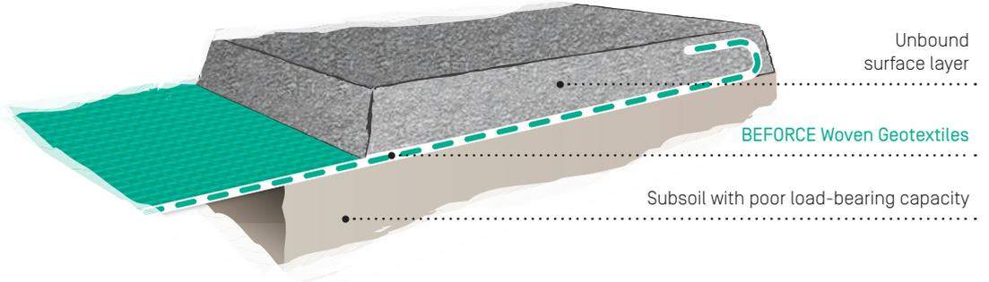
Separating and reinforcing a layer of replaced soil to improve the load-bearing capacity of the formation layer and to support vehicular traffic during the construction phase
