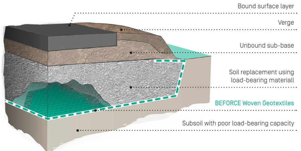
Reinforced foundation bed as a bearing layer for pipelines
