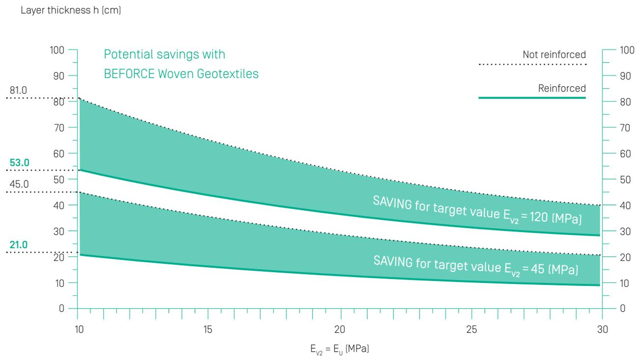
Example, based on a modulus of deformation  $E_u = 10$  MPa
