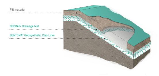
Construction method with weather-sensitive sealing element and a seepage layer
