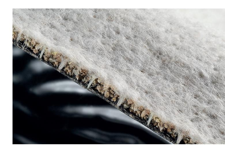
BENTOMAT GDA CL is the perfect solution when it comes to greater depths of standing water, because the flow through geosynthetic clay liners increases at higher hydraulic gradients. By adding an PE membrane, this effect is significantly impeded without having to forgo the benefits of a bentonite mat.
