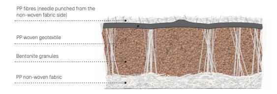
BENTOMAT GDA CL has been specially developed for applications with particularly stringent requirements in terms of sealing performance. This innovative product incorporates an PE membrane that is bonded across the whole area of the bentonite mat to create a multi-layer product. The bonded membrane provides additional protection against unwanted drying out and against root penetration.
