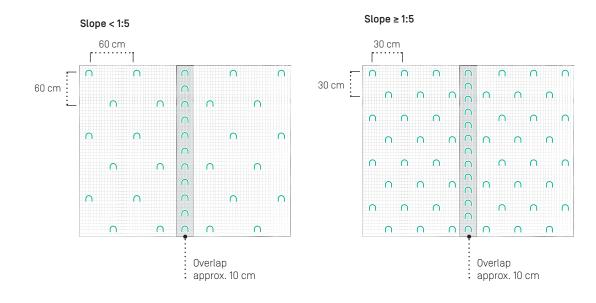
The overlap must be planned with the direction of the prevailing wind in mind, so that the wind does not blow directly under the edge and lift the mat.
