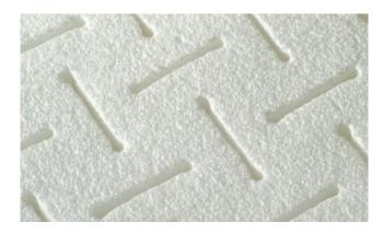
Shock Pad, laid on a suitable foundation layer, ensures excellent water permeability thanks to its cross-shaped perforations, so that the synthetic turf pitch can be used immediately after heavy rainfall.
