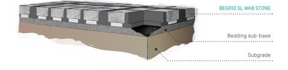
Construction method "3.5" – surfaces for cars [up to 3.5 t total weight] Pathways and cycle routes, car parks, car access roads Construction method "3.5 PLUS" – surfaces for cars and occasional HGV traffic [load class BK 0.3/BKL V/VI according to RSt0]
