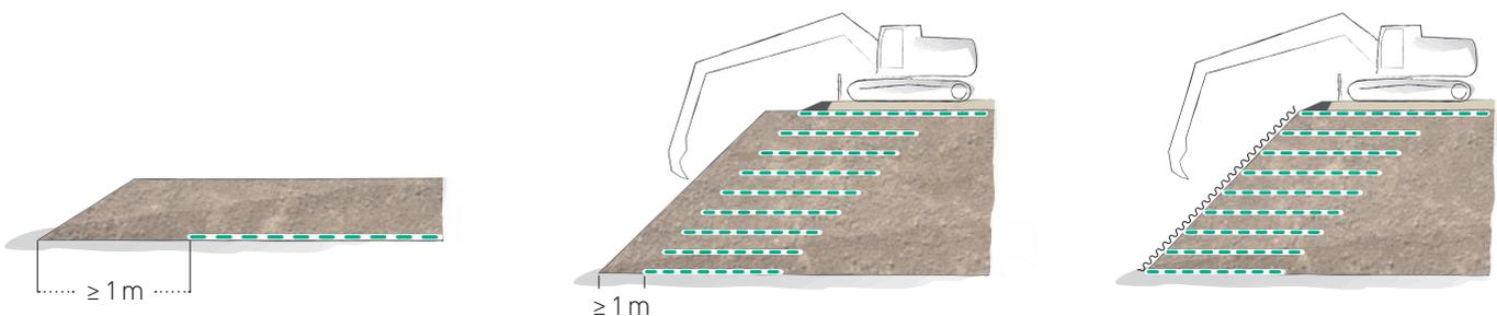
The installed layers ( $\leq 30$  cm) must be at least 1 metre wide and be compacted right up to the edges using suitable compacting machinery.
