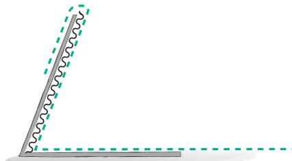
The woven or non-woven geogrid and an erosion control mat at the front are laid manually.
