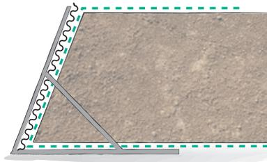
After filling and compaction, the geogrid is folded back over the soil layer.
