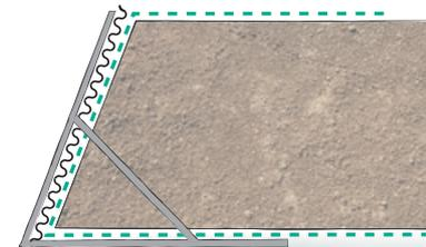
The compactable soil is laid in layers, to achieve compacted layers 40 cm thick.
