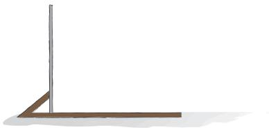
Placement of the construction formwork on the load-bearing formation.
