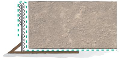
The compactable soil is laid to create compacted layers 40 cm thick.
