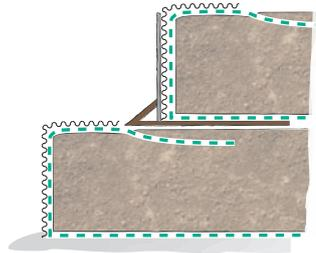
After the second layer has been laid, the formwork of the first layer is removed.
