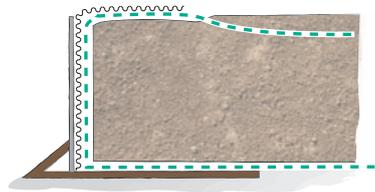
The geogrid is folded back over the soil above so that it is tied into the earthwork. The erosion control mat is embedded only up to 50 cm behind the front surface.
