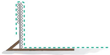
The woven or non-woven geogrid and an erosion control mat are laid.
