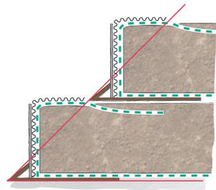
The formwork of layer 2 is set at the required embankment inclination and work continues from Step 2.
