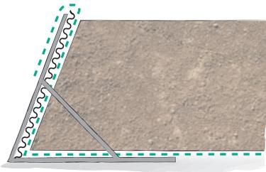
The compactable soil is laid in layers, to achieve compacted layers 40 cm thick.
