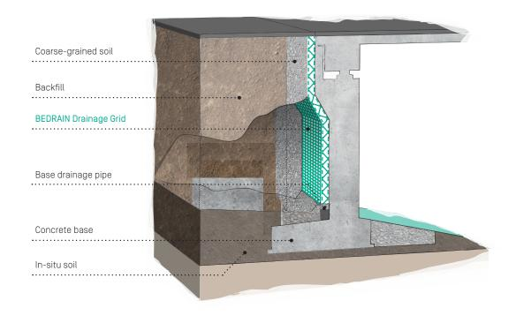
BEDRAIN Drainage Grids with a bonded geotextile on both sides meet the requirements of german standard "Was 7" for the drainage of contact surfaces between bridge abutments and backfill materials.
