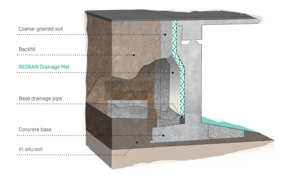
The "Riz Was 7" german standard drawing issued by the Bundesanstalt für Straßenwesen (German Federal Highway Research Institute) specifies various minimum requirements for drainage elements used for draining surfaces that come into contact with soil and for backfilling bridge structures.
