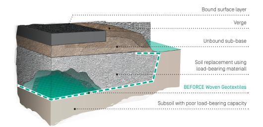
Reinforced foundation bed as a bearing layer for pipelines
