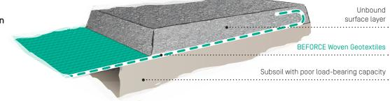
Separating and reinforcing a layer of replaced soil to improve the loadbearing capacity of the formation layer and to support vehicular traffic during the construction phase
