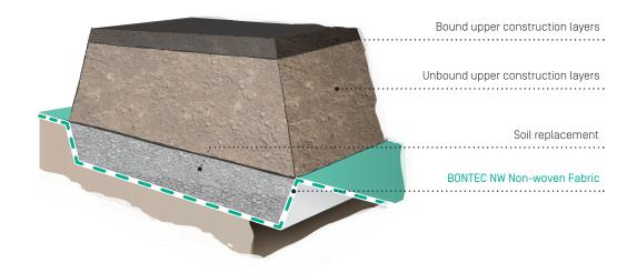
Separation layer for infilling and covering ditches and channels
