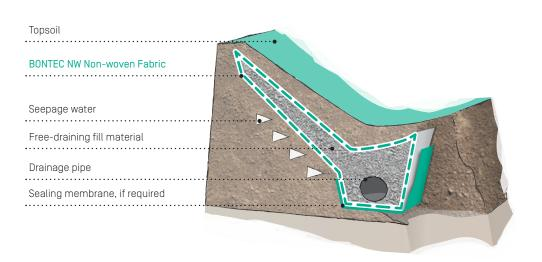
Separation and filtration layer for drainage systems
