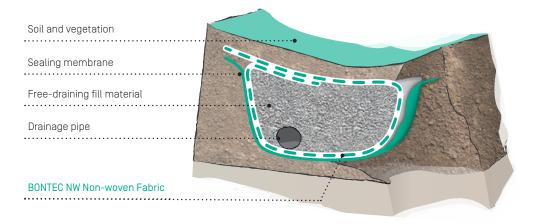
Reinstatement of a slipped embankment by installing a perforated pipe
