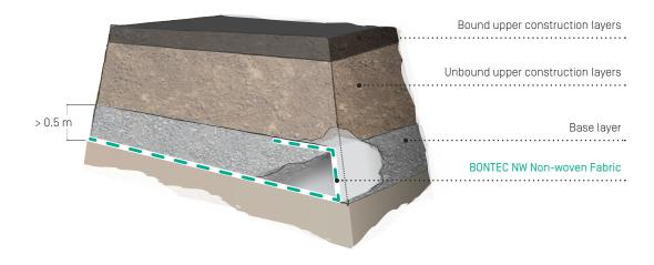
Separation layer in the case of partial soil replacement
