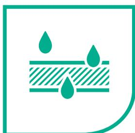
The filtration effect of a non-woven fabric becomes more important when, in addition to separation, it also has to contend with the effects of water. In such cases, the structure relies on both the separation and filtration functions of the fabric.
